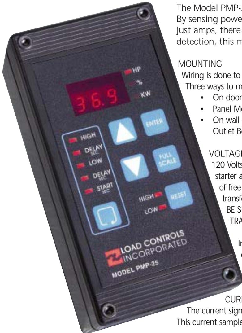
The Model PMP-25 monitors the true power going to a motor. By sensing power (volts x amps x power factor) rather than just amps, there is much greater sensitivity. For loss of load detection, this means a 10X improvement in performance.
